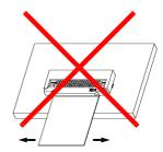
Due to the structure of the connectors, they do not have string resistance to upward pulling; therefore, support the FPC/FFC when a pulling force is applied to it.
